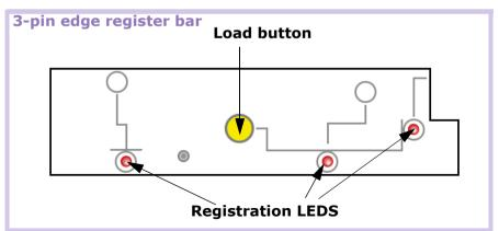
The registration LEDs help you to position the plate correctly. You use the load button to prepare the drum for plate load and to release the vacuum from the plate.
